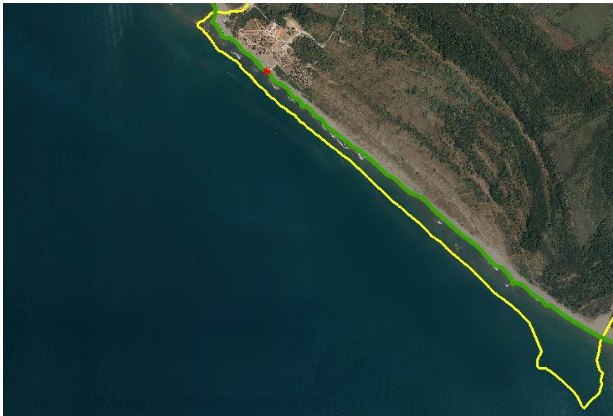
Figure 5: Diference between corrected and official coastline (official coastline is presented with yellow color)
